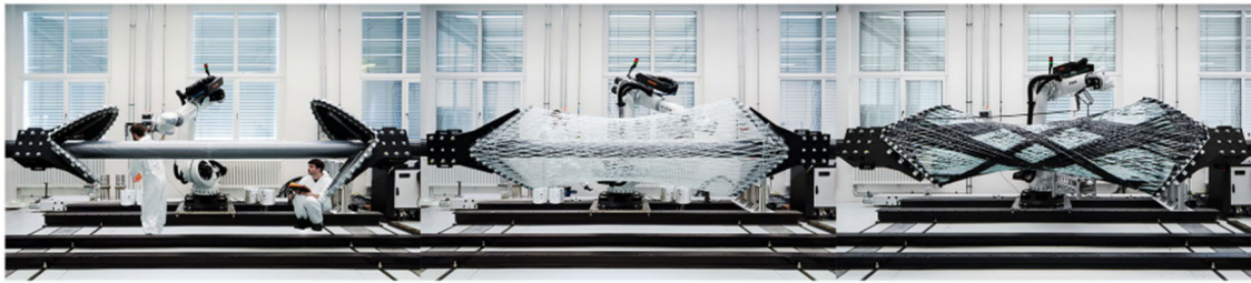
Figure 3: Fabrication sequence of a fiber reinforced composite building element. BUGA Fibre Pavilion / ICD/ITKE University of Stuttgart (2019, 09 May). ArchDaily. Accessed 08 Dec 2023. < https://www.archdaily.com/916650/buga-fibre-pavilion-icd-itke-university-of-stuttgart > ISSN 0719-8884
